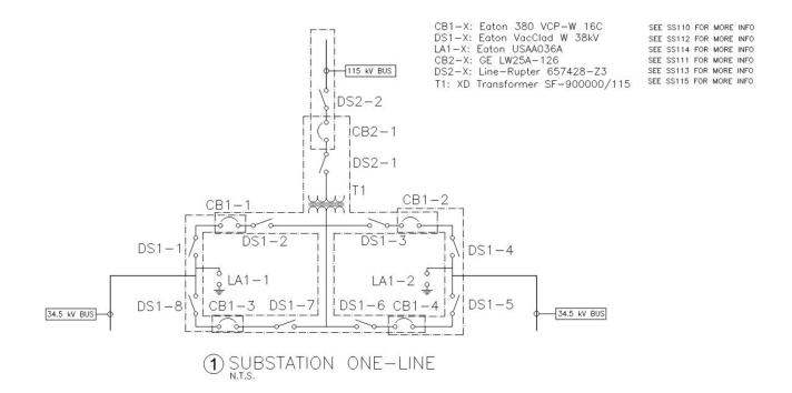
Substation One-line Diagram:
